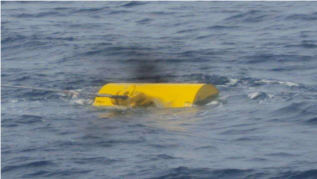
Figure 7 Buoy and hawser under tension as used in the VERSATILE MOORING SYSTEM
