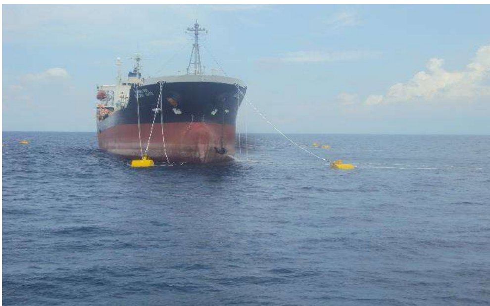
Figure 8 Small Vessel being installed and connected to the VERSATILE MOORING SYSTEM
